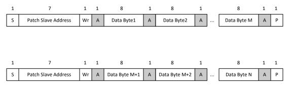
Figure 4-2. Protocol of Patch Bundle Burst Data Assuming it is Broken into Two Transactions
