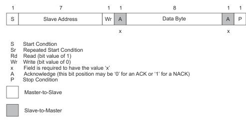
Figure 1-1. I2C Read/Write Protocol Key
