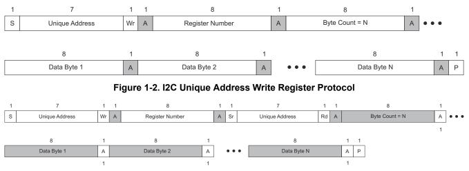
Figure 1-3. I2C Unique Address Read Register Protocol
