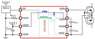
Figure 3-6. Three-Wire Mode Simplified Schematic
