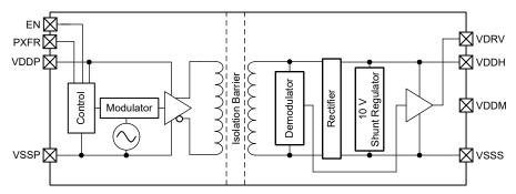
Figure 1-2. TPSI3050-Q1 Functional Block Diagram
