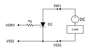
Figure 4-4. SCR for a DC Load
