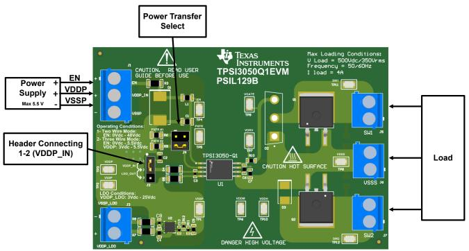
Figure 3-7. Three-Wire Mode VDDP Direct Supply
