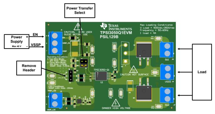
Figure 3-2. Two-Wire Mode Setup
