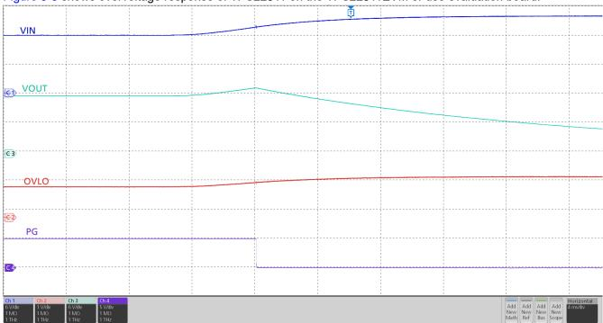
Figure 5-3. Overvoltage Protection Response of the TPS22811 Device
