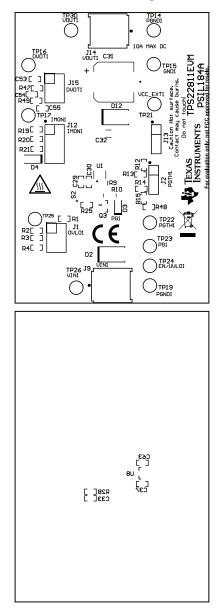
Figure 6-1. TPS22811EVM Board (a) Top Assembly (b) Bottom Assembly
