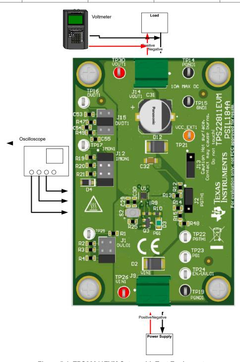
Figure 5-1. TPS22811EVM Setup with Test Equipment
