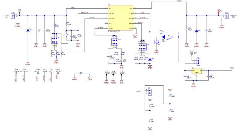
Figure 3-1. TPS22811EVM Load Switch Evaluation Board Schematic
