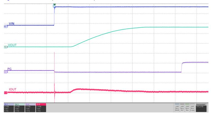
Figure 5-2. TPS22811 Output Rise Profile (VIN = 12 V, Cout = 10 uF, CdVdT = OPEN, No Load)
