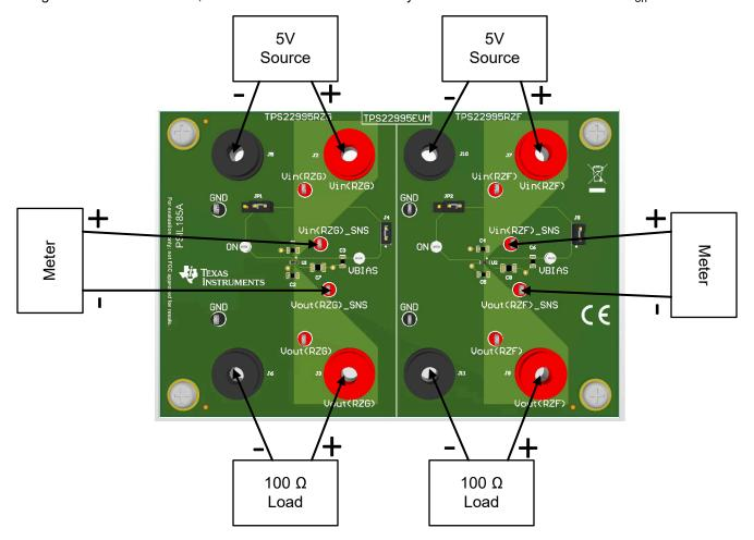
Figure 6-1. Ron Test Setup
