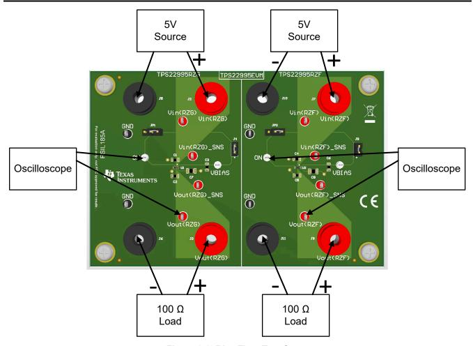
Figure 6-2. Rise Time Test Setup
