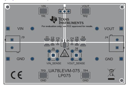
Figure 5-1. UA78LEVM-075 Top Assembly Layer and Silkscreen
