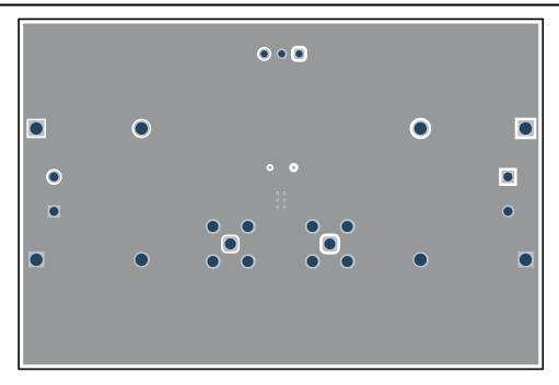
Figure 5-3. UA78LEVM-075 Bottom Layer Routing
