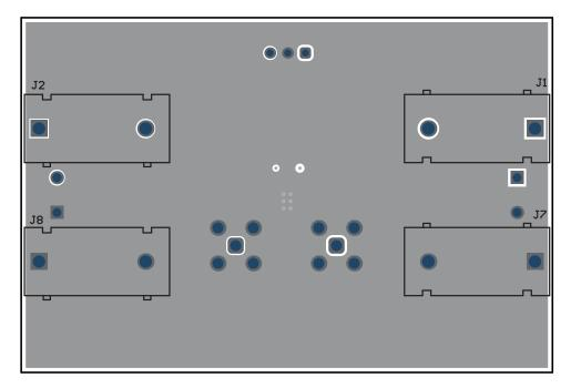
Figure 5-4. UA78LEVM-075 Bottom Assembly Layer and Silkscreen
