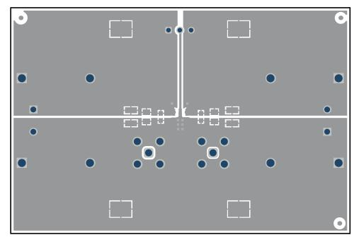
Figure 5-2. UA78LEVM-075 Top Layer Routing
