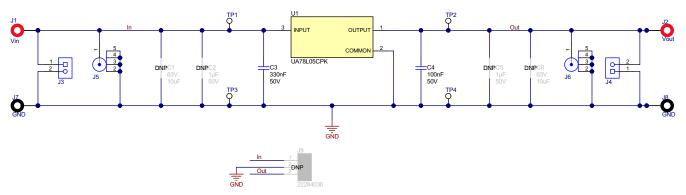
Figure 2-1. UA78LEVM-075 Schematic
