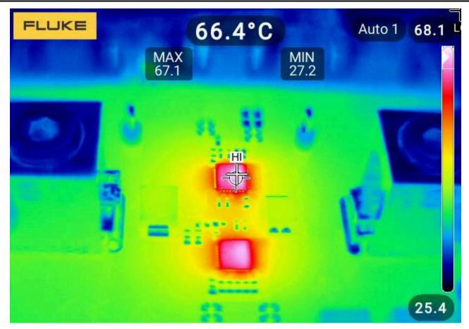
$V_{IN}$  = 12 V,  $I_{OUT}$  = 110 A,  $T_A$  = 25°C, and no external air flow
