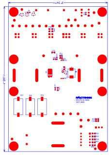
Figure 6-2. TPS25984EVM Board: Bottom Assembly
