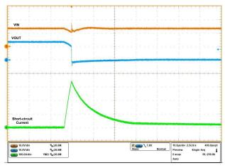
$V_{IN}$  = 12 V,  $R_{IMON}$  = 1.1 || 1.1 k $\Omega$ ,  $R_{IREF}$  = 40.2 k $\Omega$ , and  $C_{OUT}$  = 10  $\mu F$
