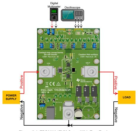
Figure 5-1. TPS25984EVM Setup With Test Equipment
