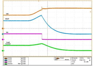
$V_{IN}$  Ramped Up from 12 V to 18 V,  $C_{OUT}$  = 470  $\mu$ F, and  $R_{LOAD}$  = 1.2  $\Omega$
