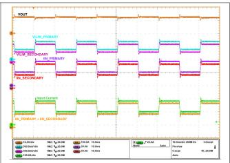
$V_{IN}$  = 12 V,  $C_{ITIMER}$  = 22 nF,  $C_{OUT}$  = 470 μF,  $R_{IMON}$  = 1.1 || 1.1 kΩ,  $R_{IREF}$  = 40.2 kΩ,  $I_{OUT}$  ramped from 98 A to 180 A then 98 A within 10 ms
