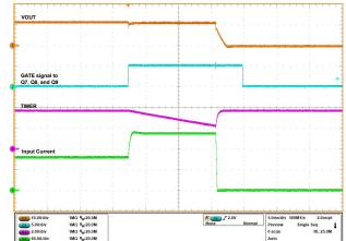
$V_{IN}$  = 12 V,  $C_{ITIMER}$  = 22 nF,  $C_{OUT}$  = 470  $\mu$ F,  $R_{IMON}$  = 1.1  $\parallel$  1.1 k $\Omega$ , R<sub>IREF</sub> = 40.2 k $\Omega$ , I<sub>OUT (Steady-State)</sub> = 100 A, and  $I_{OUT (Transient)} = 69 A for 18 ms$
