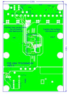
Figure 6-8. TPS25984EVM Board: Layer 5 (Signal)
