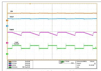
$V_{IN}$  = 12 V,  $C_{ITIMER}$  = 22 nF,  $C_{OUT}$  = 470  $\mu\text{F},\,R_{IMON}$  = 1.1  $\parallel$  1.1  $k\Omega,\,R_{IREF}$  = 40.2  $k\Omega,\,I_{OUT}$  ramped from 100 A to 175 A then 100 A within 10 ms
