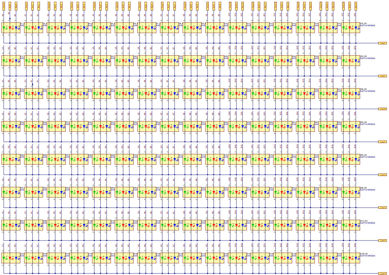
Figure 5-4. LP5890EVM Schematic (4 of 4)
