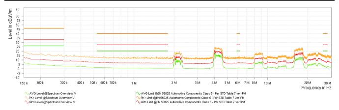
Figure 5-14. CISPR 25 Radiated Emissions: 150 kHz to 30 MHz, MONOPOLE
