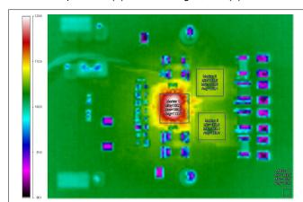
Figure 5-24. Infrared Thermal Image: VIN = 12 V,  $T_{AMB}$  = 85°C, 200LFM, IOUT = 8 A
