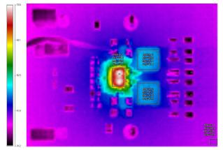
Figure 5-20. Infrared Thermal Image: VIN = 12 V,  $T_{AMB}$  = 25°C, 200LFM, IOUT = 12 A
