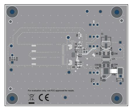
Figure 6-3. Bottom Component View
