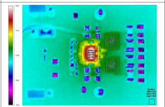
Figure 5-23. Infrared Thermal Image: VIN = 12 V,  $T_{AMB}$  = 85°C, 200LFM, IOUT = 10 A
