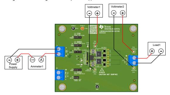
Figure 4-1. EVM Test Setup
