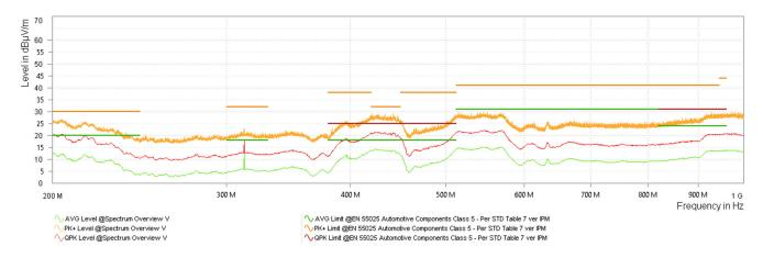
Figure 5-16. CISPR 25 Radiated Emissions: 200 MHz to 1 GHz, LOG
