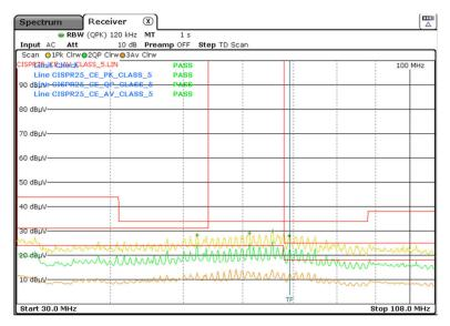
Figure 5-13. CISPR 25 Conducted Emissions: 30 MHz to 108 MHz
