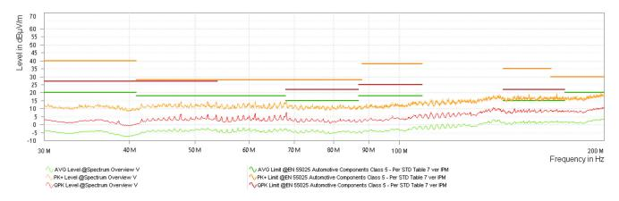
Figure 5-15. CISPR 25 Radiated Emissions: 30 MHz to 200 MHz, BICON
