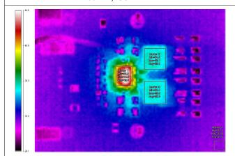
Figure 5-22. Infrared Thermal Image: VIN = 12 V,  $T_{AMB}$  = 25°C, 200LFM, IOUT = 8 A
