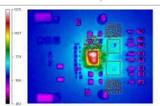
Figure 5-19. Infrared Thermal Image: VIN = 24 V, IOUT = 10 A
