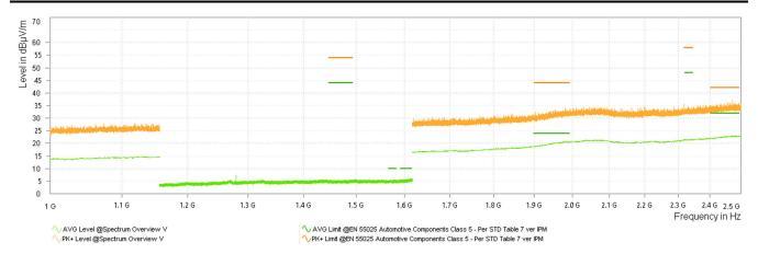
Figure 5-17. CISPR 25 Radiated Emissions: 1 GHz to 2.5 GHz, HORN
