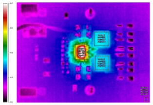
Figure 5-21. Infrared Thermal Image: VIN = 12 V,  $T_{AMB}$  = 25°C, 200LFM, IOUT = 10 A
