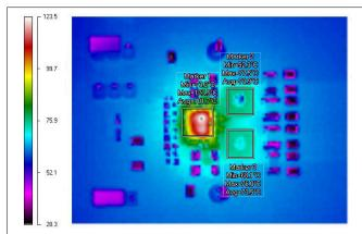
Figure 5-18. Infrared Thermal Image: VIN = 12 V, IOUT = 12 A
