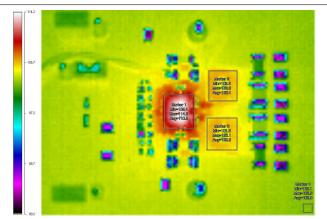
Figure 5-25. Infrared Thermal Image: VIN = 12 V,  $T_{AMB}$  = 85°C, 200LFM, IOUT = 6 A
