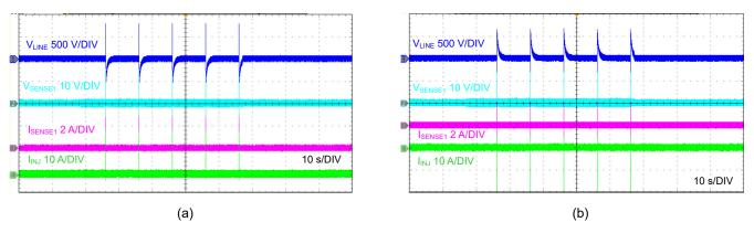
Figure 3-5. IEC 61000-4-5 Surge, 6-kV Repetitive Strike at 10-Second Intervals – Positive (a), Negative (b)
