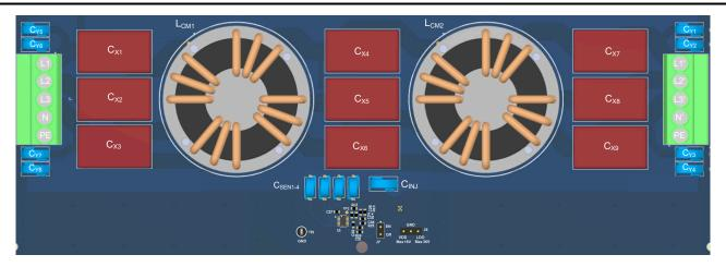
Figure 2-3. Filter Component Placement Example
