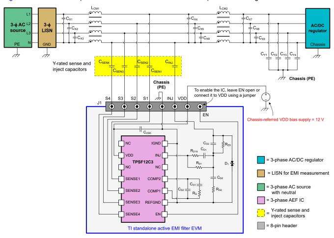
Figure 2-2. EVM Setup Schematic for High-Voltage Testing With a Three-Phase AC/DC Regulator
