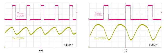
Figure 3-7. TPSF12C3 INJ (pin 13) Voltage With CM Stimulus Signal Applied – 100 kHz (a), 65 kHz (b)
