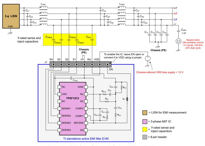
Figure 2-4. EVM Setup Schematic for Low-Voltage Testing
