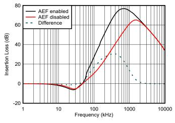
Figure 3-2. Typical CM Insertion Loss with AEF Enabled and Disabled
