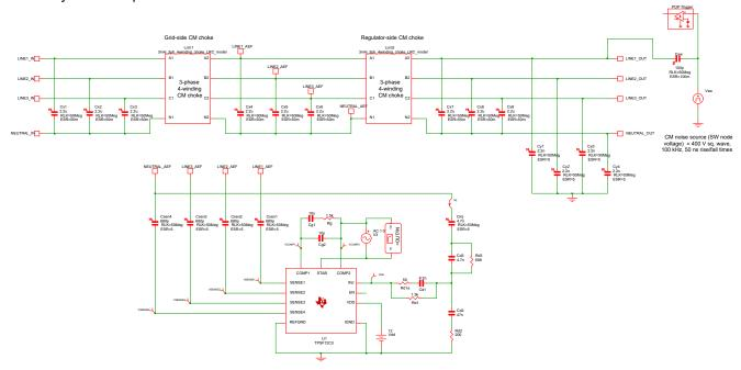
Figure 2-6. SIMPLIS Simulation Schematic of an Active Filter Circuit Using the TPSF12C3
