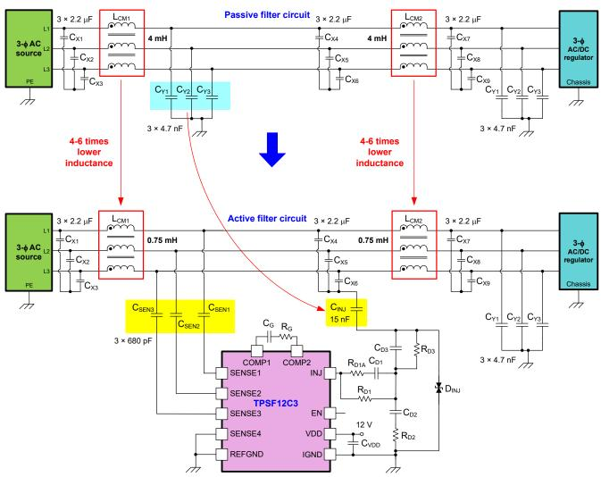
Figure 1-2. Three-Phase, Three-Wire Passive and Active Filter Schematics
