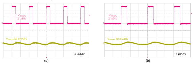
Figure 3-6. TPSF12C3 SENSE (pin 4) Voltage With CM Stimulus Signal Applied – 100 kHz (a), 65 kHz (b)
