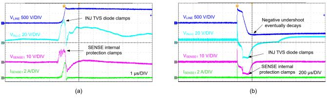
Figure 3-3. IEC 61000-4-5 Positive Surge, 6-kV Single Strike – 1 µs/div (a), 200 µs/div (b)
