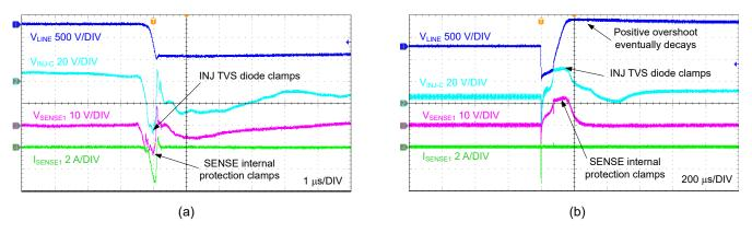
Figure 3-4. IEC 61000-4-5 Negative Surge, 6-kV Single Strike - 1 µs/div (a), 200 µs/div (b)
