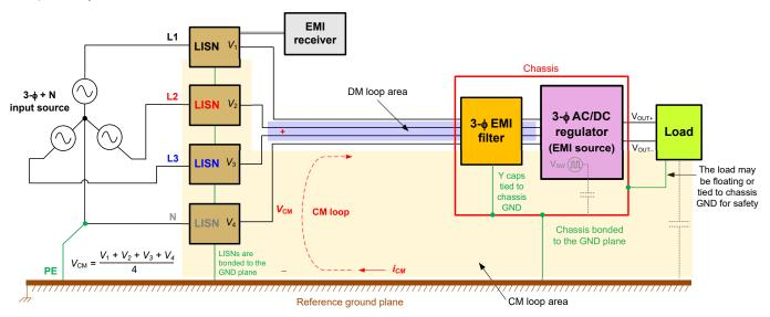
Figure 2-1. EMI Measurement Setup for a Three-Phase System
