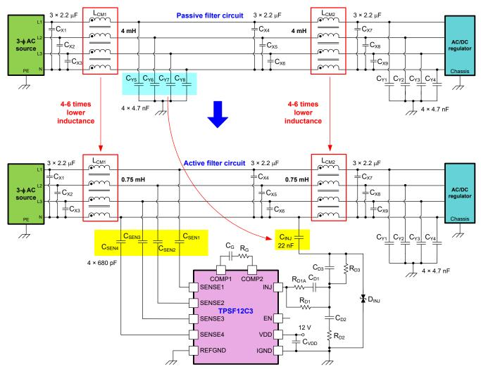
Figure 1-1. Three-Phase, Four-Wire Passive and Active Filter Schematics
