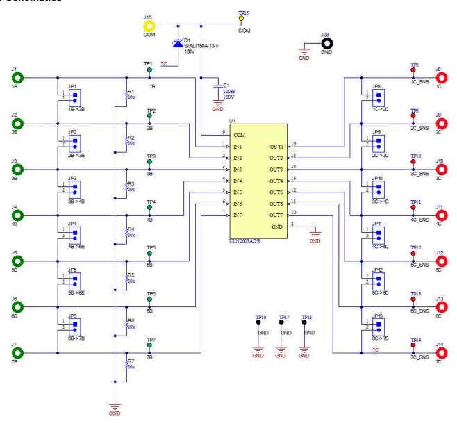
Figure 3-1. ULN2003ADEVM Schematic Drawing
