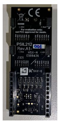
Figure 2-1. TPS25730EVM Bottom View of the Jumper Locations
