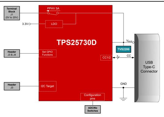
Figure 1-1. TPS25730EVM Block Diagram
