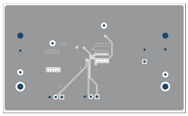
Figure 3-5. Inner Layer 2 Layout
