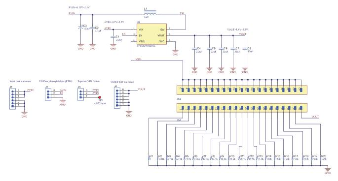
Figure 3-1. TPS61299EVM-016 Schematic
