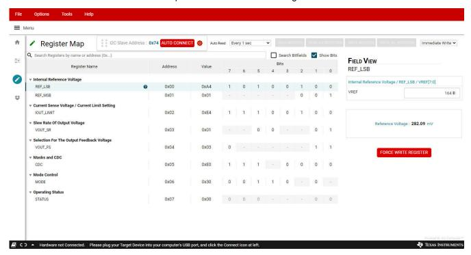
Figure 3-7. GUI Register Map Screen
