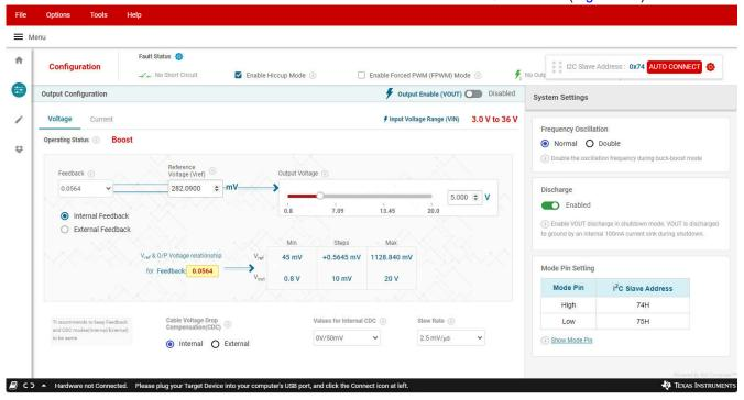
Figure 3-4. GUI User Interface of TPS55289Q1EVM-011
