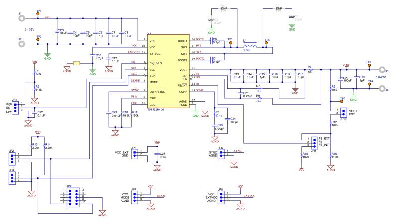
Figure 4-1. TPS55289Q1EVM-011 Schematic
