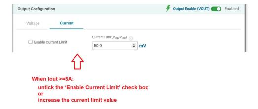
Figure 3-6. Output Current Limit Point Setting
