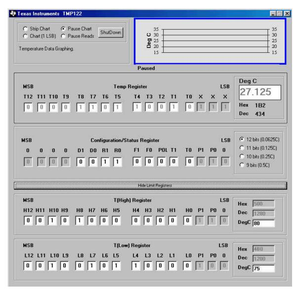
? User can set the Limit values by typing the values in either register directly or in the boxes that are located right of the registers. It is always desirable that value of T(Low) Register to be lower than T(High) Register.
