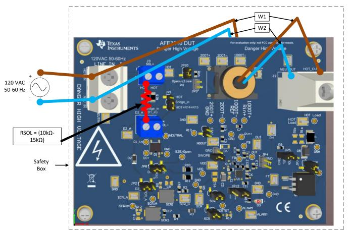
Figure 2. AFE3010EVM and Hardware Setup
