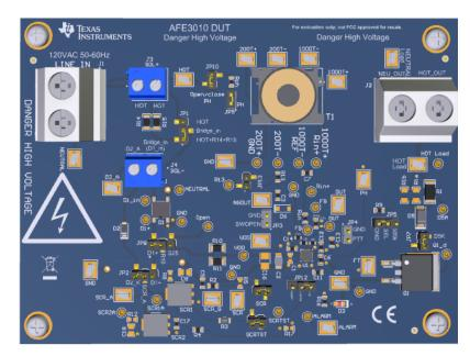
This user's guide describes the characteristics, operation, and use of the AFE3010 evaluation module (EVM). This EVM is designed to evaluate the performance of the AFE3010 as a ground-fault circuit interrupter IC with self-tests. Throughout this document, the terms evaluation board, evaluation module, and EVM are synonymous with the AFE3010EVM. This document also includes a schematic, reference printed-circuit board (PCB) layouts, and a complete bill of materials (BOM).
