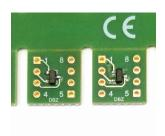
**Step 1:** Solder IC(s) to adapter PCB. Also solder any necessary decoupling capacitor needed for the device. Refer to the device data sheet for appropriate decoupling capacitor values. ICs may be hand-soldered or attached with IR or hot air reflow techniques.
