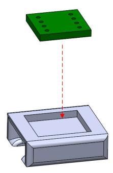
Figure 3-8. Install PCB to SENS093\_Slider
