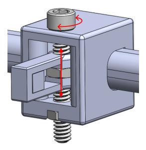
Figure 3-12. Vertical Adjustment Screw
