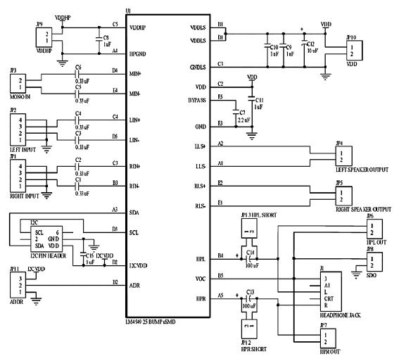
Figure 2. LM4949 Demoboard Schematic
