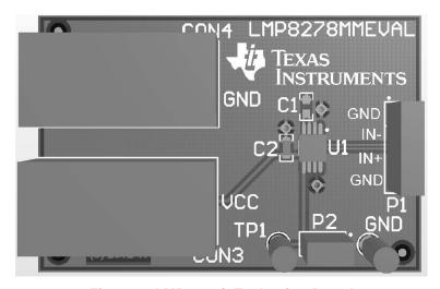
Figure 1. LMP8278Q Evaluation Board
