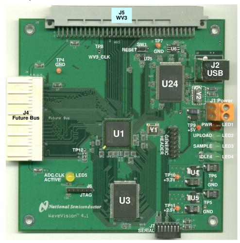
Figure 1 WaveVision4 (version 4.1) Data Capture Board Layout
