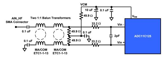
Figure 3. Analog Input Network of ADC11C125HFEB: F<sub>IN</sub> > 150 MHz
