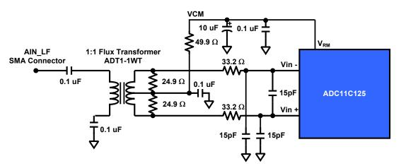
Figure 2. Analog Input Network of ADC11C125LFEB: F<sub>IN</sub> < 150 MHz
