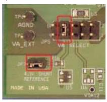
Figure 5: LM4050 Jumper Configuration
