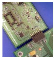
Figure 6: WV4 to ADC121C02XEB Connection
