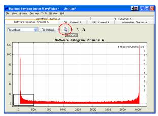
Figure 12: Software Histogram: Sine Wave Input
