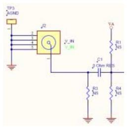
Figure 2: DC Coupled Input Configuration
