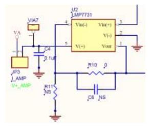
Figure 4: Input Buffer Configuration
