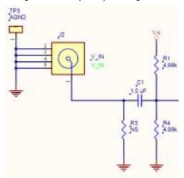
Figure 3: AC Coupled Input Configuration
