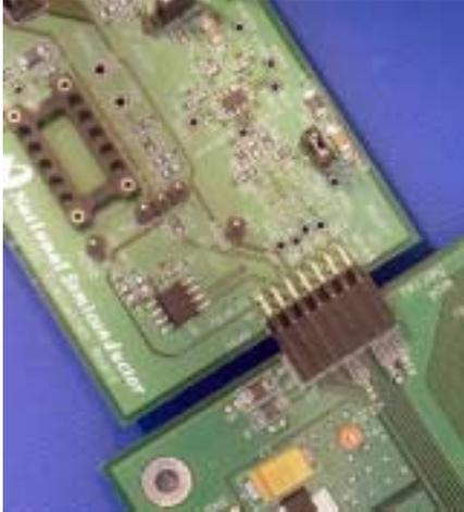
**Figure 6: WV4 to ADC121C02XEB Connection**
