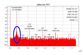
Figure 3. Jitter causes a spreading around the input signal, as well as undesirable signal spurs.
