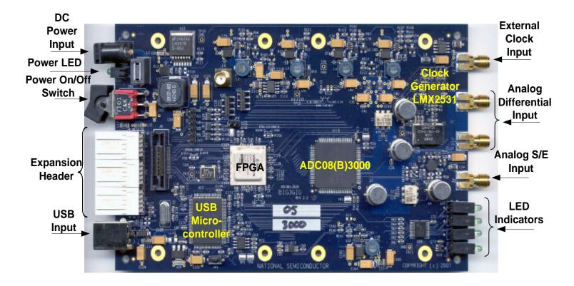
Figure 1. Input/Output Connection and Board Overview
