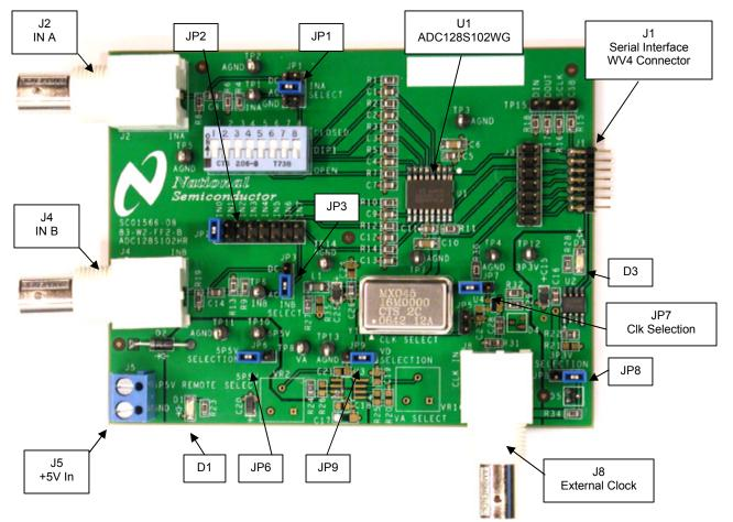
Figure 1: Component and Test Point Locations
