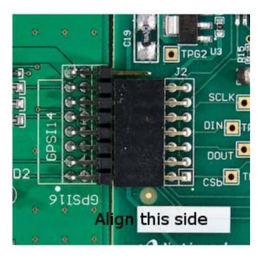
Figure 2: DAC161S055 Eval board connected to SPUSI board.
