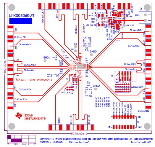
Figure 6: Top Side, Layer #1 (Not to scale)
