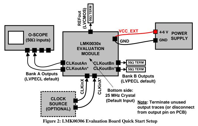
1. Verify the output mode control switches, S1[1:5], match the states shown in Table 1 to reflect the default output clock interfaces configured on the EVM.
