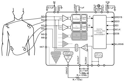
Figure 7: 3-LEAD ECG Connection
