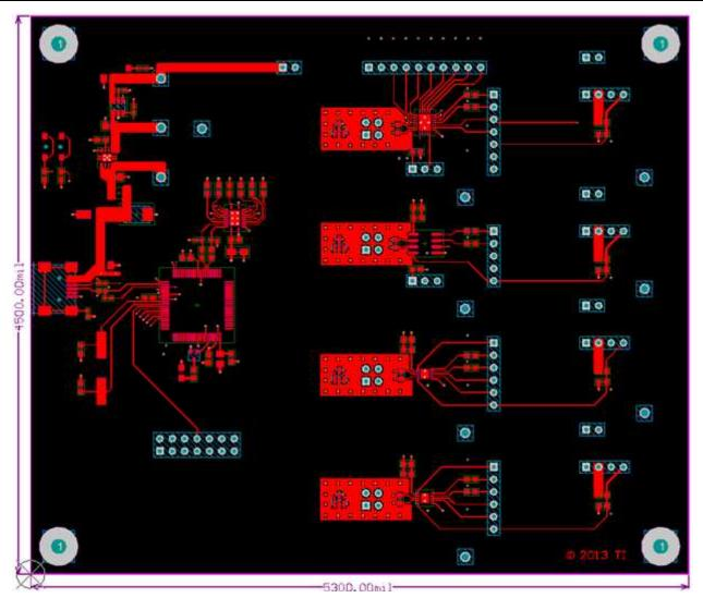
Figure 32. Top Layer Routing
