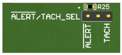
Figure 4. LM63 ALERT/TACH Select Jumper
