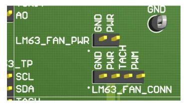
Figure 14. LM63 Fan Connector
