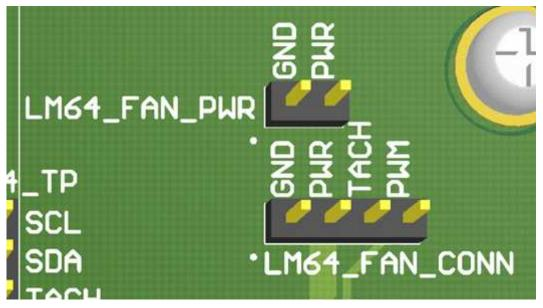
Figure 15. LM64 Fan Connector
