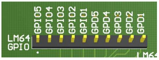
Figure 7. LM64 GPIO Test Points
