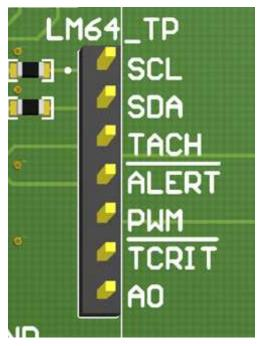
Figure 5. LM64 Test Points
