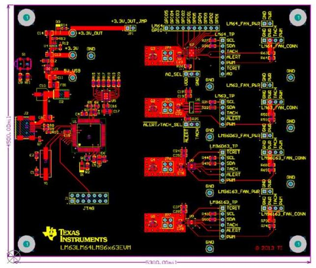
Figure 31. Top Assembly Layer
