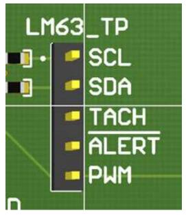
Figure 3. LM63 Test Points
