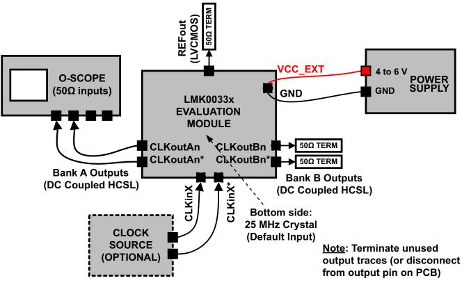
Figure 1. LMK00338 Evaluation Board Quick Start Setup
