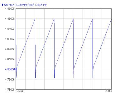
Figure 10. Continuous Sawtooth Ramp Example
