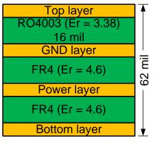
Figure 19. PCB Layer Stack-up
