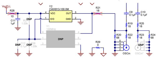
Figure 31. Reference Clock Input Configuration
