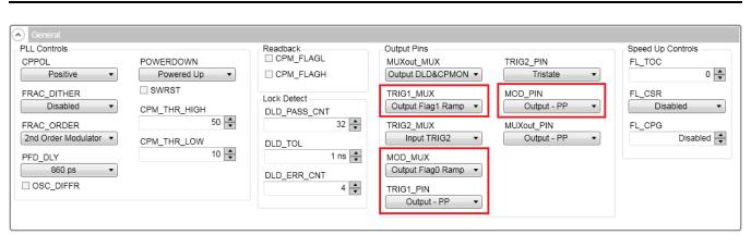
Figure 12. Flag Out Pins Configuration
