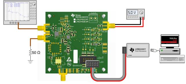
Figure 1. EVM Connection Diagram
