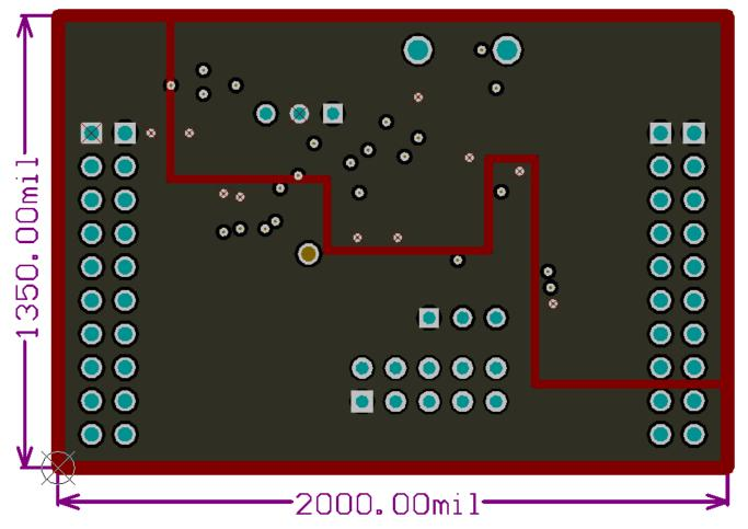
Figure 4-3. Power Layer Routing
