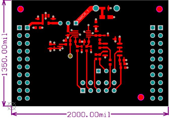
Figure 4-2. Top Layer Routing
