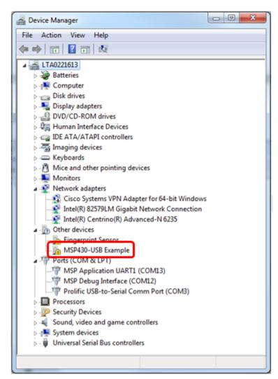
Figure 2-4. Driver Not Installed
