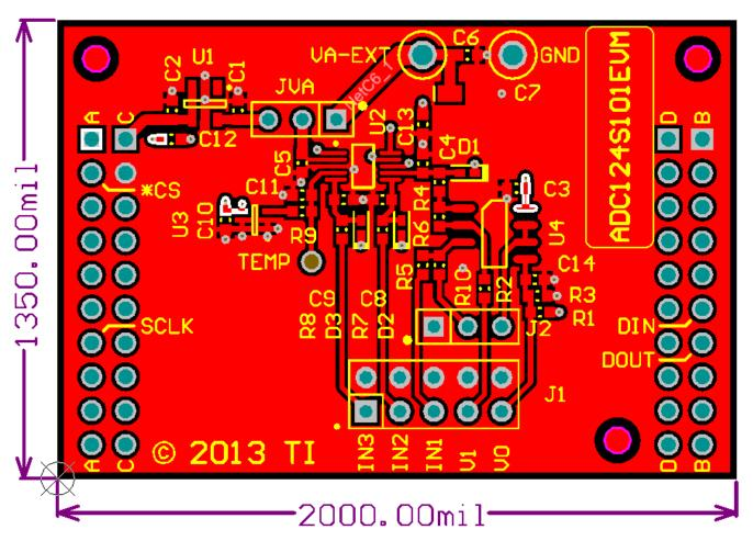
Figure 4-1. Top Assembly Layer
