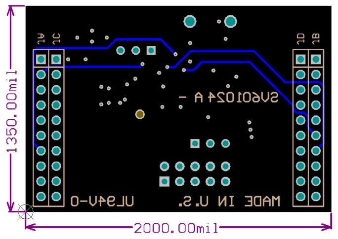
Figure 4-5. Bottom Layer Routing
