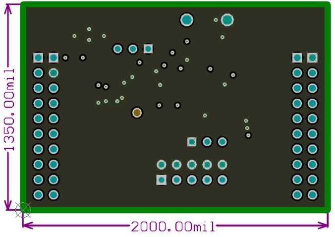
Figure 4-4. Ground Layer Routing
