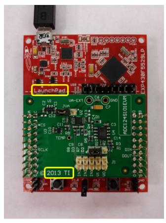
Figure 3-1. ADC124S101EVM Attached to MSP430
