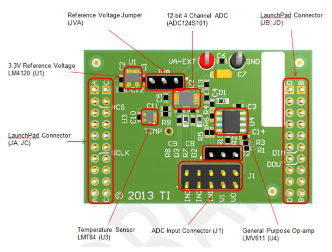
Figure 1-1. ADC124S101EVM Evaluation Board
