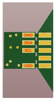
Figure 12. HDC1080EVM Pads for I2C and Supply of the Smaller Sensor Section
