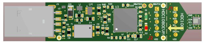
Figure 10. HDC1080EVM µC and Sensor Sections
