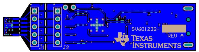
Figure 55. Bottom Layer Routing
