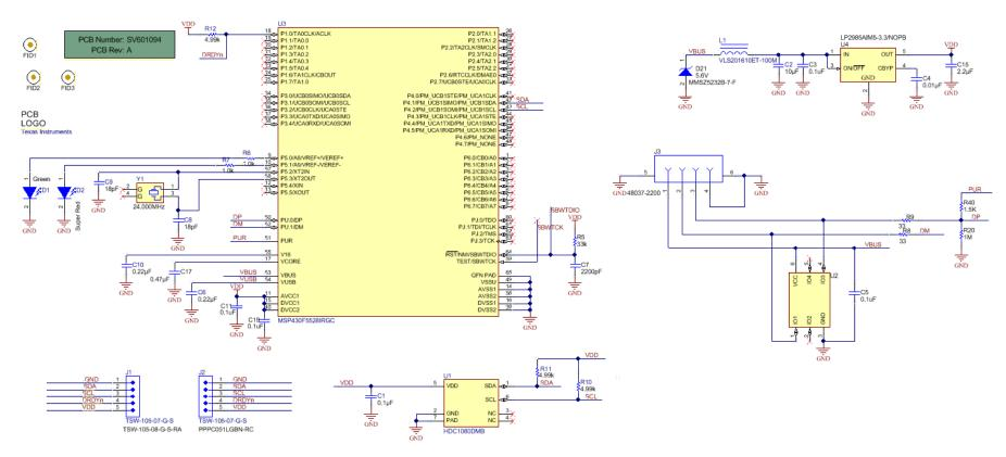
Figure 56. HDC1080EVM Schematic
