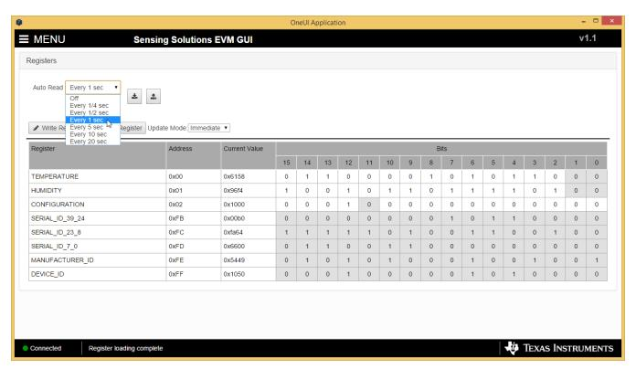
Figure 21. Selecting Auto-Read Interval on Register Page
