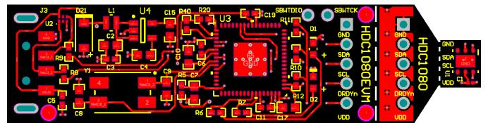
Figure 54. Top Layer Routing
