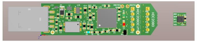
Figure 13. HDC2080EVM : PC Interface and Smaller Sensor Module
