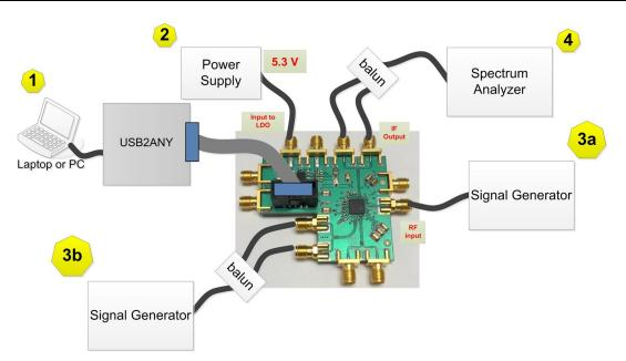
Figure 2. Setup Diagram for LMX8410L in External LO Mode
