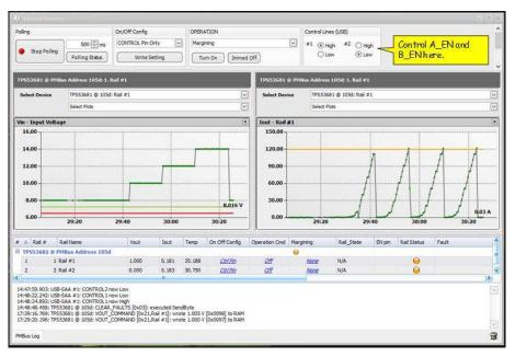
Figure 7. System Monitor Window: Control Lines
