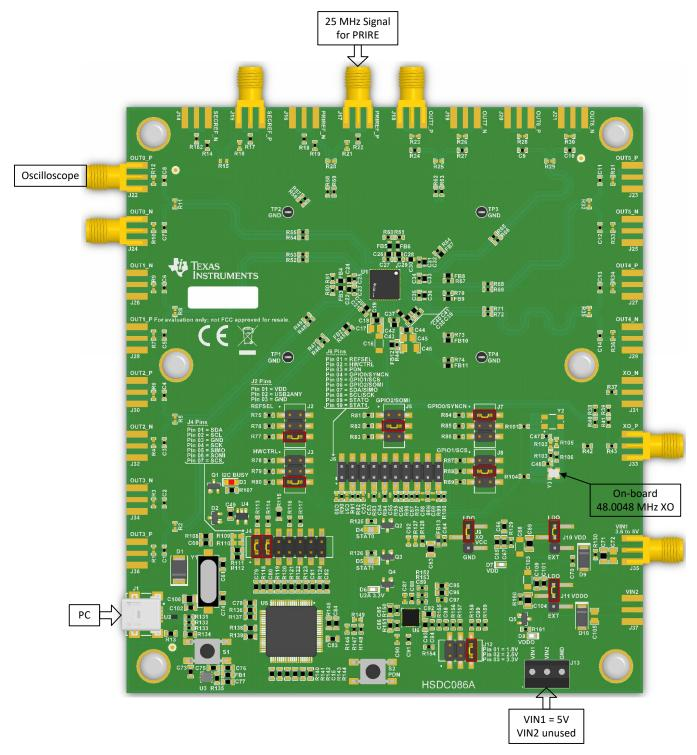
Figure 1. LMK05318B EVM with Default Jumper Settings
