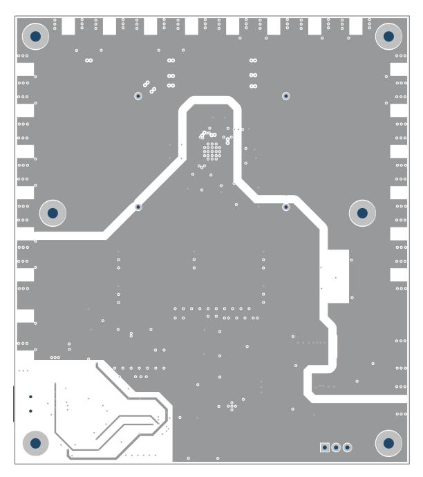
Figure 14. Layer 4 - Power Routing
