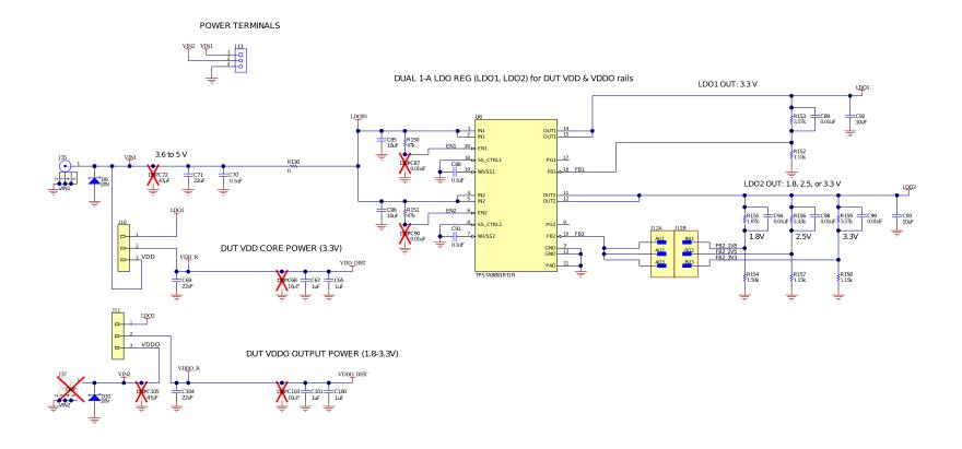
Figure 2. Schematic 1 - Power Supply
