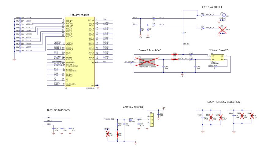
Figure 4. Schematic 3 - LMK05318B and XO Input Interfaces
