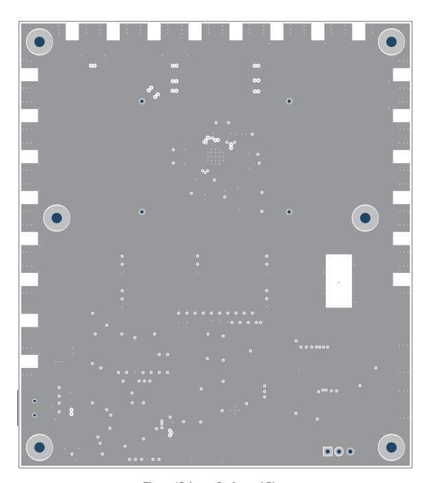
Figure 15. Layer 5 - Ground Plane
