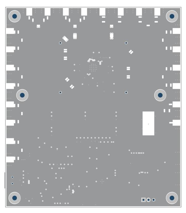
Figure 12. Layer 2 - Ground Plane
