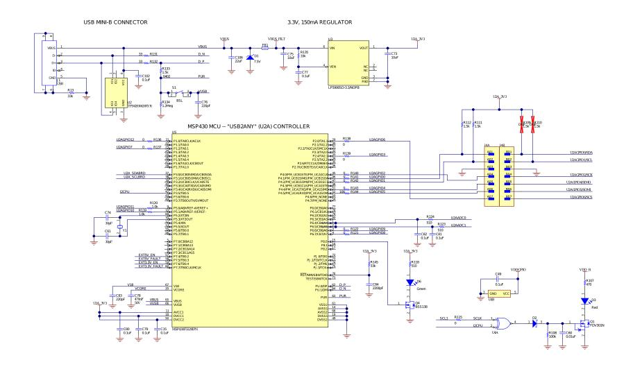
Figure 9. Schematic 8 - USB MCU and I<sup>2</sup>C/SPI Jumper Block
