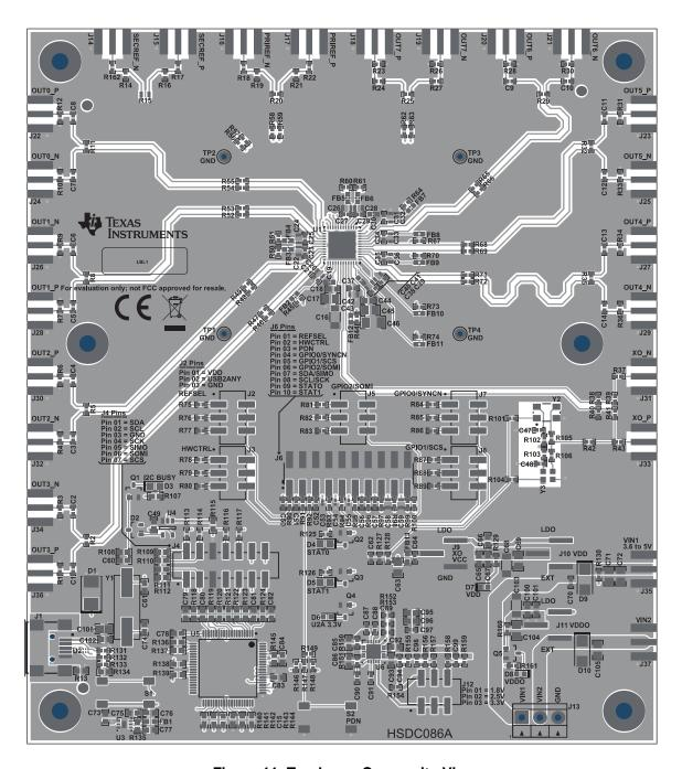
Figure 11. Top Layer Composite View
