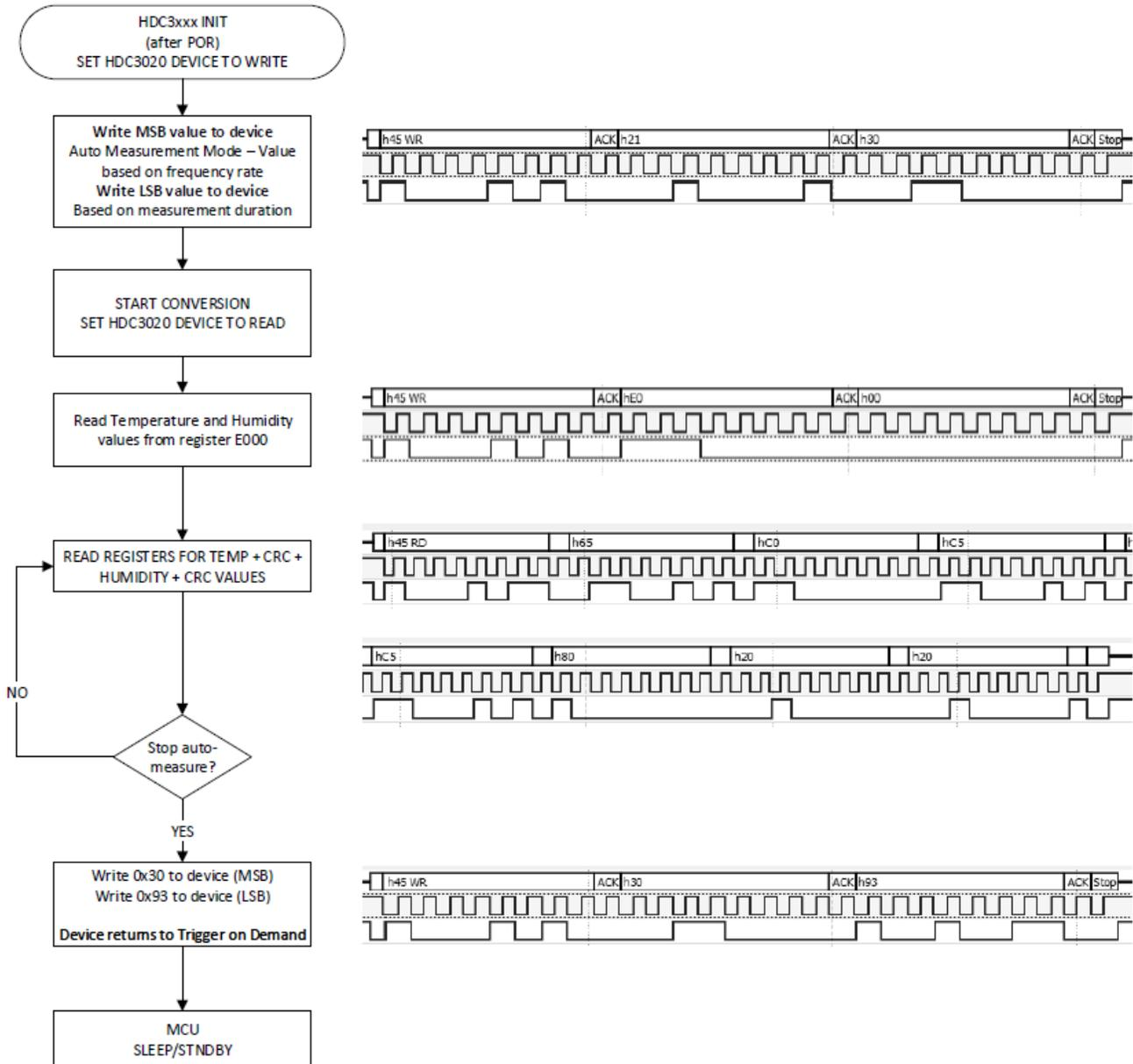
Figure 3-2. Flowchart for Auto-Measurement Mode
