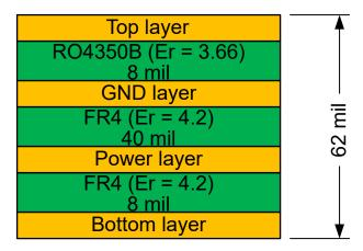
Figure 5-1. PCB Layer Stack-Up
