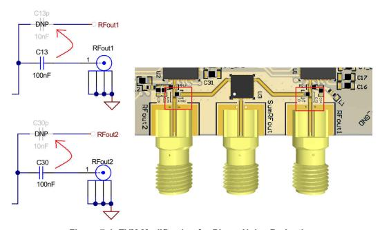
Figure 7-1. EVM Modification for Phase Noise Reduction
