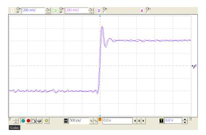
Figure 3-4. Output Phases After Synchronization
