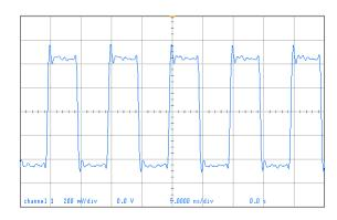
Figure 9-3. Default Output Phase Nosie
