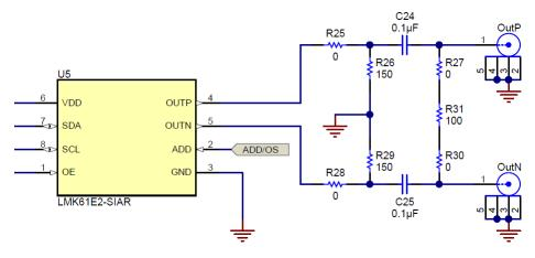
Figure 9-2. Output Termination Schematic
