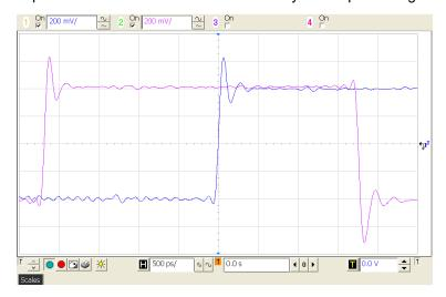
Figure 3-2. Output Phases Before Synchronization
