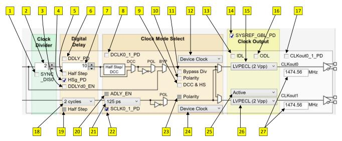
Figure 2-2. Clock Outputs Page Description Diagram
