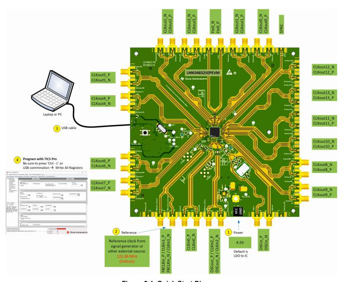
Figure 2-1. Quick Start Diagram
