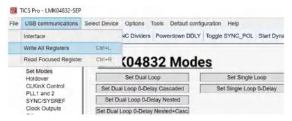
Figure 5-2. Loading the Device
