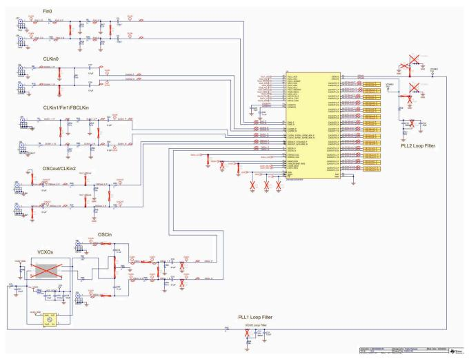
Figure 8-1. Schematic - LMK04832-SEP
