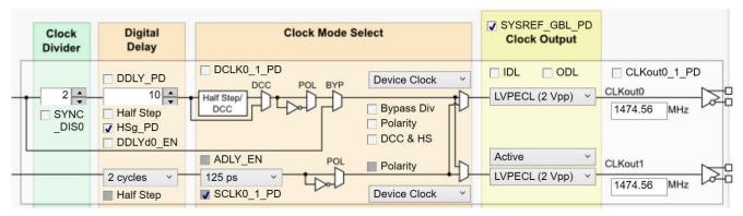
Figure 5-4. Setting Digital Delay, Clock Divider, Analog Delay, and Output Format
