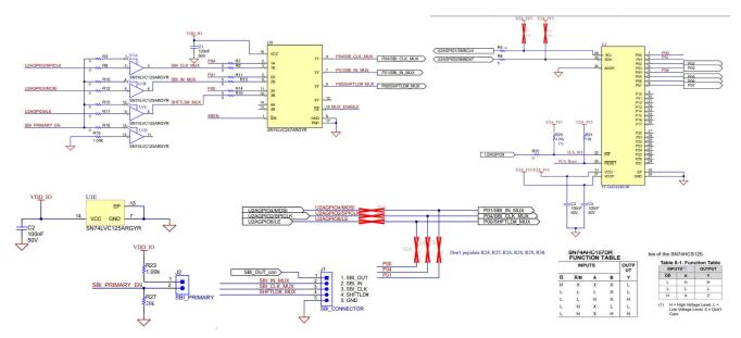
Figure 5-8. I/O Expander, MUX, and Buffer Used for SBI and OE Pin Control
