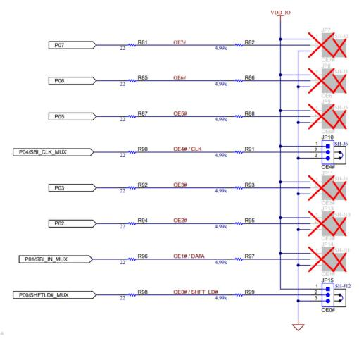
Figure 5-4. Output Enable Pins (OE#)
