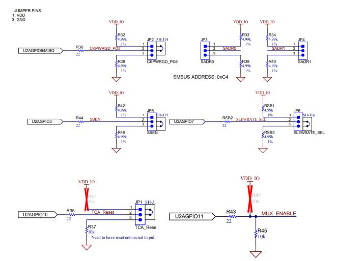
Figure 5-5. Logic I/O Jumpers
