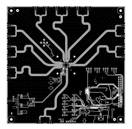
Figure 5-10. Top Layer (CLKIN / CLKOUT Signals)
