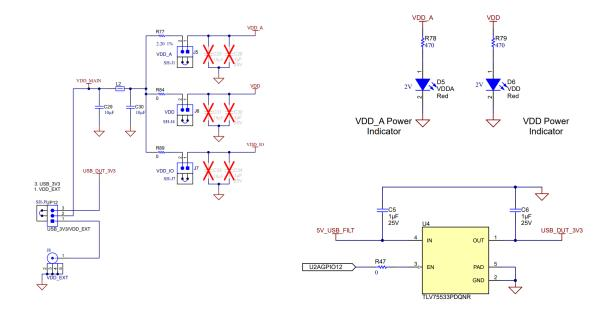
Figure 5-1. Power Supply (External and USB option)
