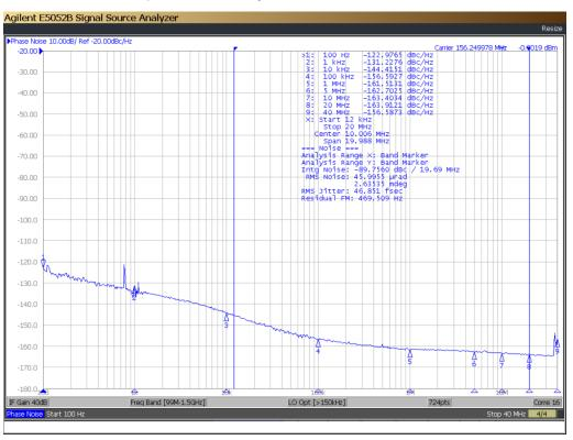
Figure 4-1. LMKDB1108 Output Clock Phase Noise
