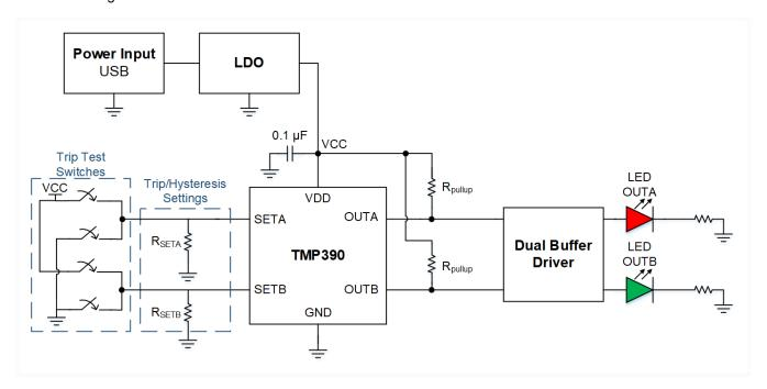
Figure 4. TMP390 Evaluation Board Block Diagram
