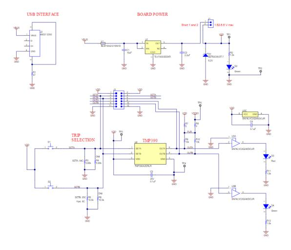
Figure 6. TMP390 Evaluation Board Schematic
