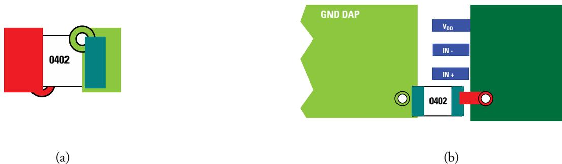
Figures 5-8a and 5-8b. Typical Decoupling Capacitor Layouts
