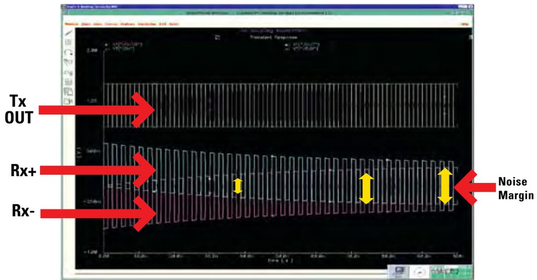
Figure 4-3. AC-Coupled Differential Pair at Startup
