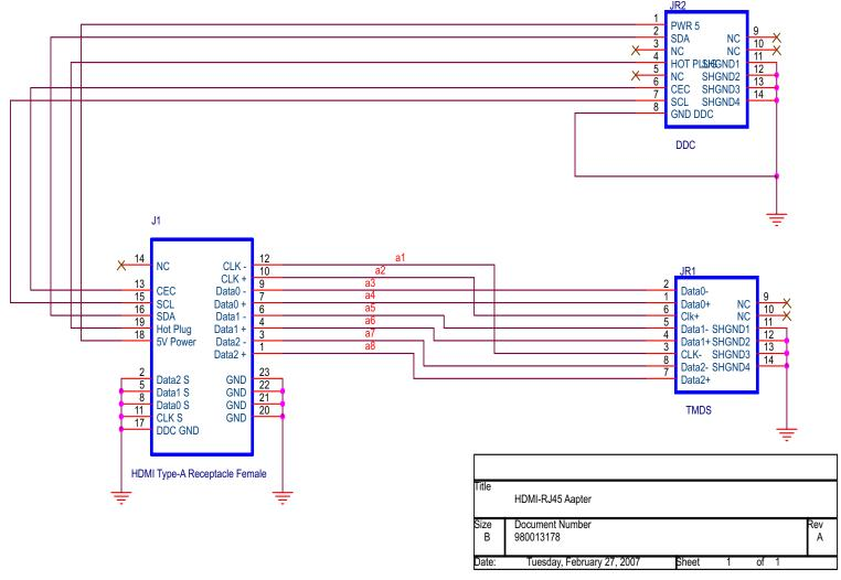
Figure 2. Schematic (Passive Adapter Board)
