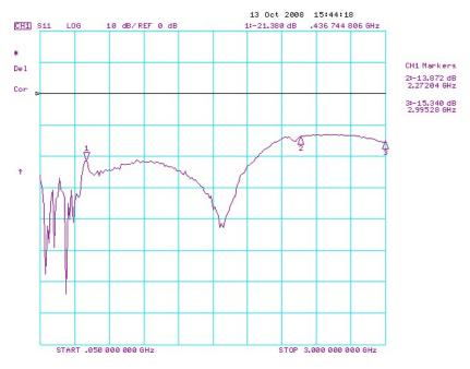
FIGURE 4. Output Return Loss (ORL) on SDO (plus)
