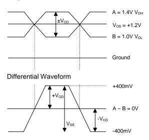
Figure 5: Single-ended and Differential Waveforms
