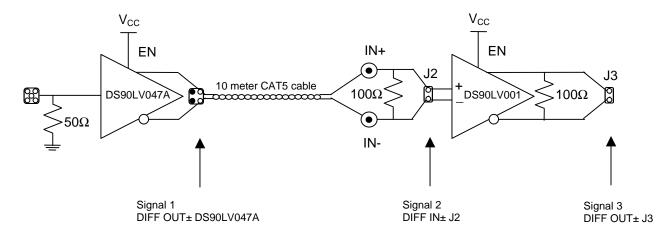
Figure 6: Input and Output LVDS Signals in Cable Repeater Application
