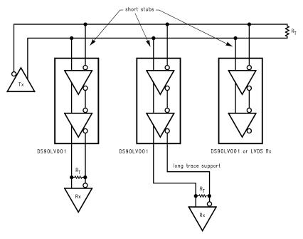
Figure 2: Backplane Stub-Hider Application
