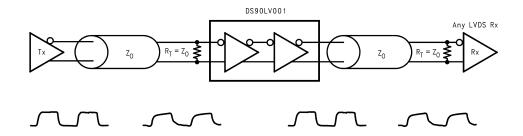
Figure 1: Cable Repeater Application
