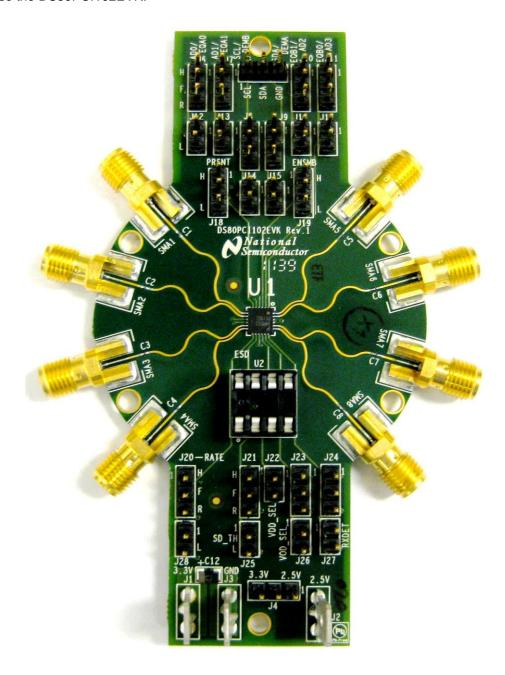
Figure 1: DS80PCI102EVK Evaluation Board
