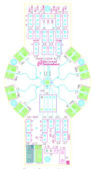
Figure 3: Top Assembly Layer
