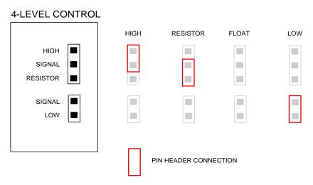
Figure 2: 4-Level IO Control on EVK
