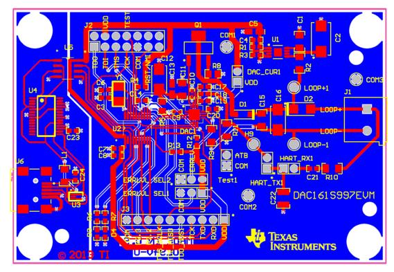
Figure 10. Top Assembly Layer
