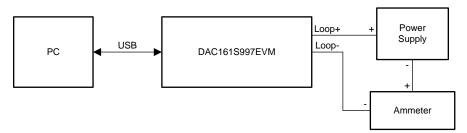
Figure 2. EVM Connection Diagram
