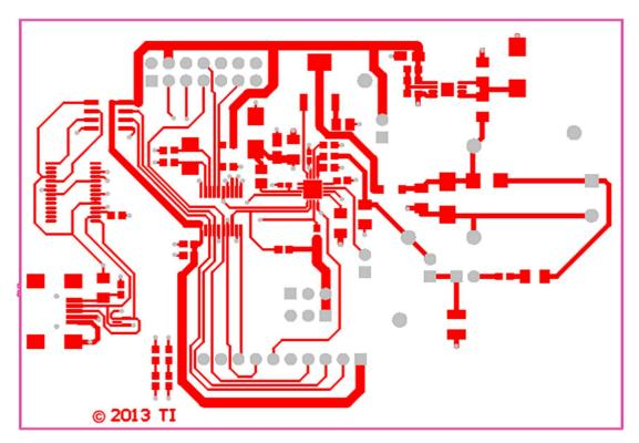
Figure 11. Top Layer Routing
