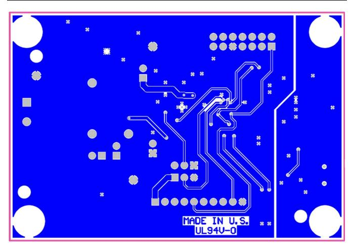
Figure 12. Bottom Layer Routing
