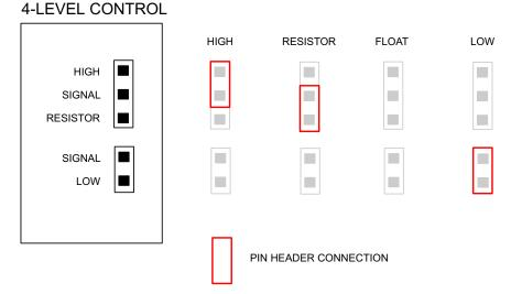
Figure 2. 4-Level IO Control on EVM
