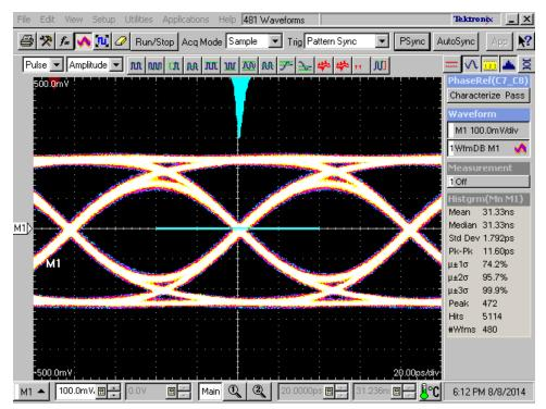
Figure 3. 12 Gbps Eye Diagram at SCOPE in SETUP1
